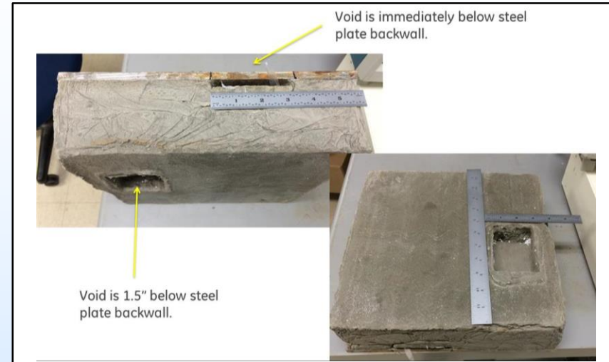
Concrete phantom with air void defects
